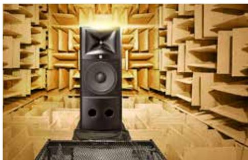
JBL research facilities feature multiple application-specific anechoic testing chambers and showcase our “Speaker Shuffler” – the only one of its kind – which allows rapid and precise re-positioning of speaker systems in the exact same precise position, for unrivaled accuracy in A/B testing. Our rigorous, uncompromising testing methodologies result in continuous performance breakthroughs and ensure that JBL customers worldwide can always work with confidence.
