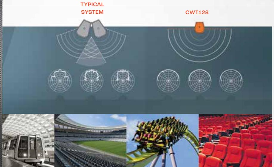
To provide high quality, full bandwidth sound evenly dispersed across a coverage area greater than 100°, often two speaker systems are mounted and played to achieve wider horizontal coverage. But this approach produces interference where the coverage patterns overlap resulting in uneven sound fields and compromised intelligibility.
