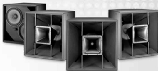
The PD500 Series is a line of loudspeaker systems consisting of four horn-loaded 380mm (15") 2-way systems and one dual 380mm (15") subwoofer.
