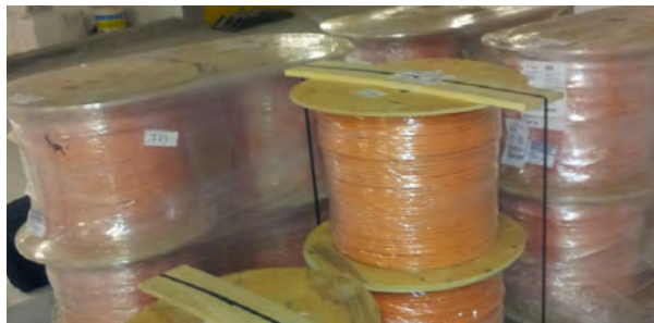
Copper cable stored in good conditions
