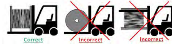
Correct lifting procedure
